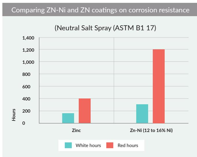
White hours represent the time it took to corrode the plating. (Zinc degrades into a white rust.) Red hours represent the time it took to corrode the substrate, which usually forms red rust.
