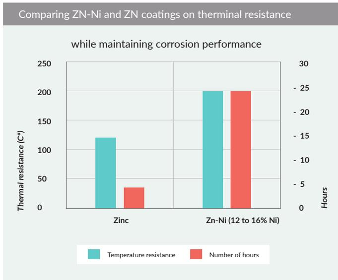
As European and American regulators require longer life for vehicles, Zn-Ni provides a significant advantage for manufacturers by protecting parts from corrosion. Similarly, as aging infrastructure is replaced or repaired, the use of these coatings on fasteners and other structural elements helps ensure longer life for those structures.
